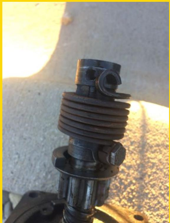
Wally was having trouble with his brake lights and I lost a bolt on the bendix of the starter.
