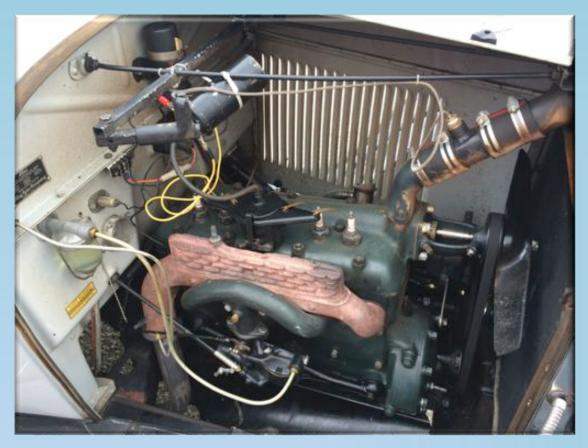
The last day of the trip at the hotel Ken and Arlene are having problems shifting their trans. Gears are clashing no matter what they do. Phil checks out the clutch pedal linkage, and it seemed to be adjusted properly. In the meantime, Ken's car won't start and now it is raining. Again a weak spark! We hang another coil from the hood rod and use jumper wires. We then pull started his car and got it running. Once it warmed up, he said it is running real nicely.
